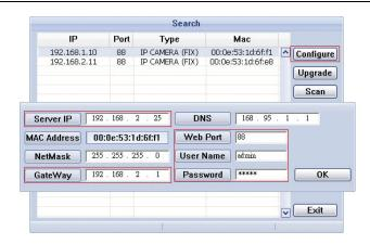
Step3: Select the IP address you want to configure, and click "Configure" to show the IP setting page, and change the IP address, gateway and port number.
