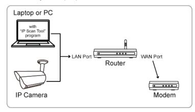
Devices connected with a RJ45 network cable
