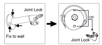
Step3: Fasten the camera with the joint lock to the bracket.
