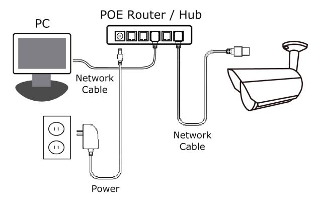
■ When your router / hub doesn't support POE connection (An optional POE connected required)
