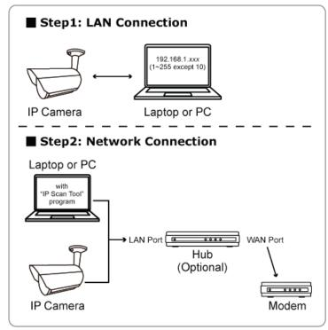
→ Devices connected with a RJ45 network cable
