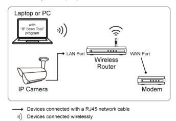
Step2: Open "IPScan.exe" (\(\mathbb{c}\)) to search your camera. The default IP address of the camera is **192.168.1.10**. If you connect two or more cameras to the wireless router, "IPScan" will list many cameras with different IP addresses after searching. To know which camera you're configuring, you may identify each with its unique MAC address.
